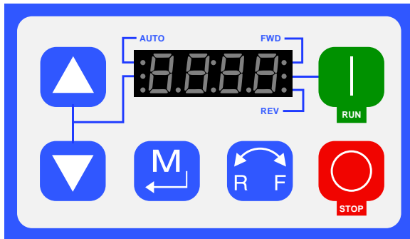
Figure 15 VFD Control Panel
