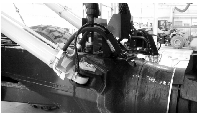
FIG. 116: Hoist cylinder; right side
