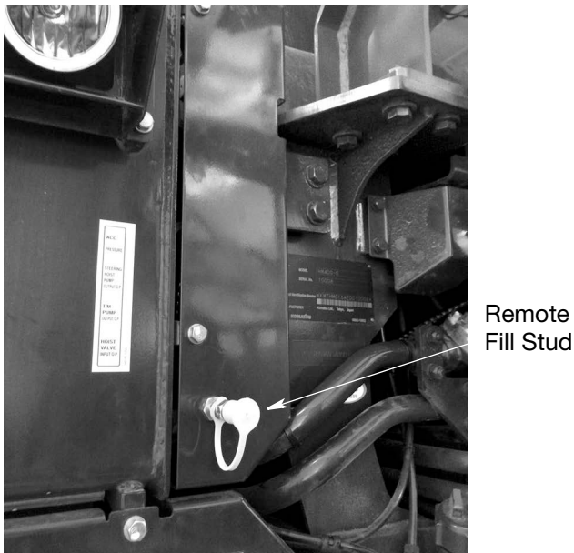
FIG. 52: Remote Fill Stud installed on HM400-5
