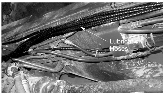
FIG. 108: Hoses running along left side dump body frame rail to back of truck dump bed on HM300-5.
