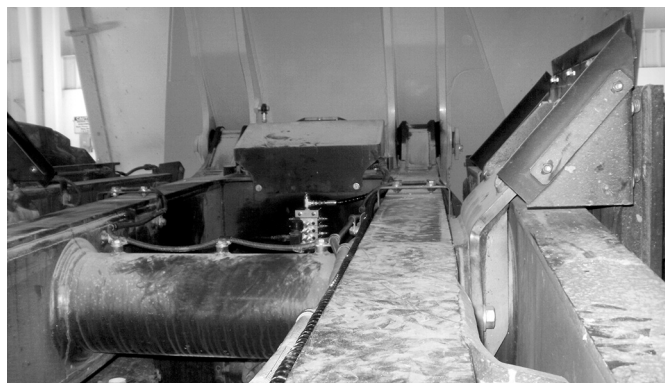
FIG. 110: Master to Rear Secondary Valve supply hose. Routed along left side dump body frame rail to divider valve on HM300-5.
