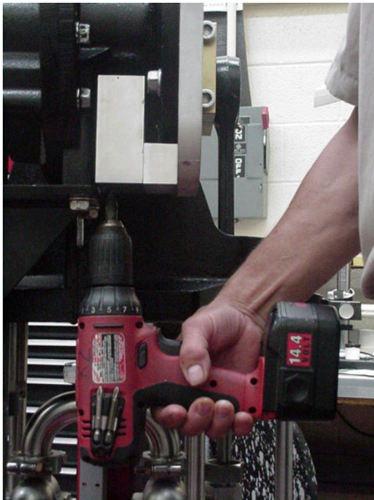
FIG. 3. Drill the Hole for the Position Sensor
