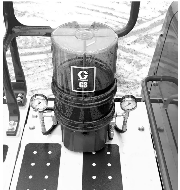
FIG. 32: G3 Pump installed on PC360-11/PC390-11/PC490-11 Models
