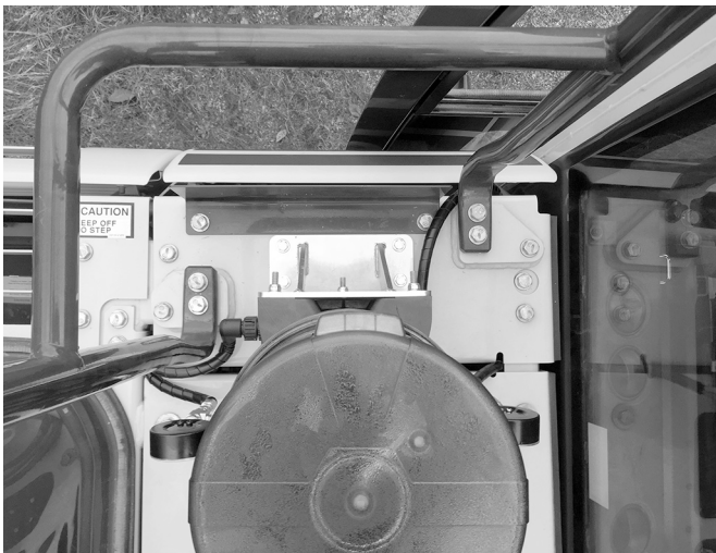
FIG. 31: G3 Pump installed on left side of PC210-11/PC240-11/PC290-11 Models
